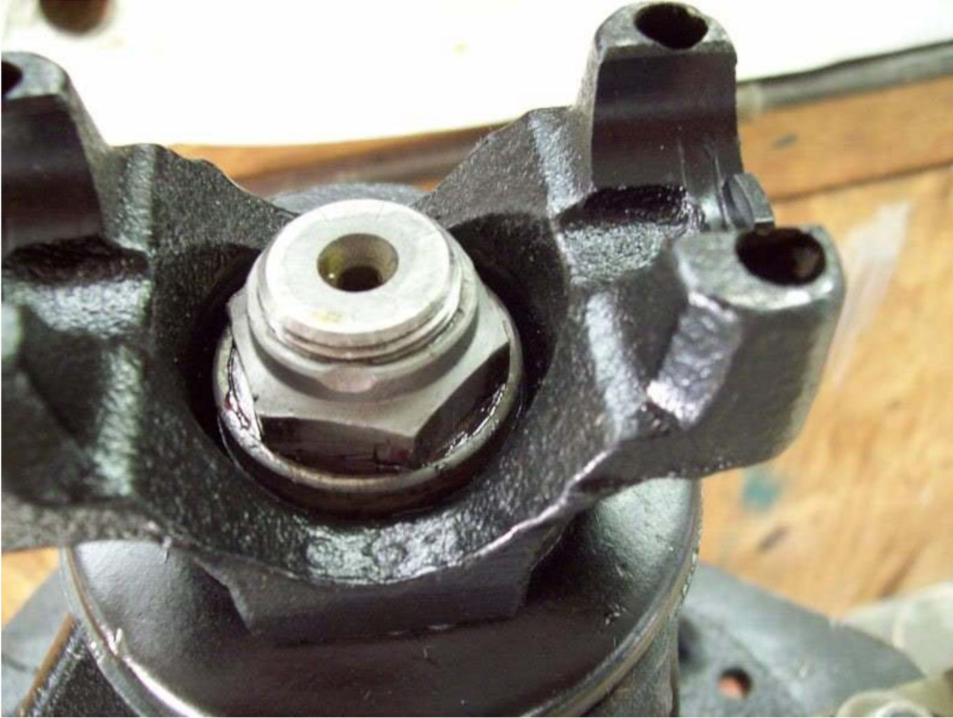
When I first setup the pinion with the new crush sleeve, BEFORE installing the new seal, I only tighten the nut to achieve about 20in/lb preload on the pinion bearings. Once the seal is installed and the yoke, washer and nut is finally installed, I also use gasket sealer on the washer and nut, then finish tightening the pinion nut to achieve the 25in/lbs specified in the rearend manual.
