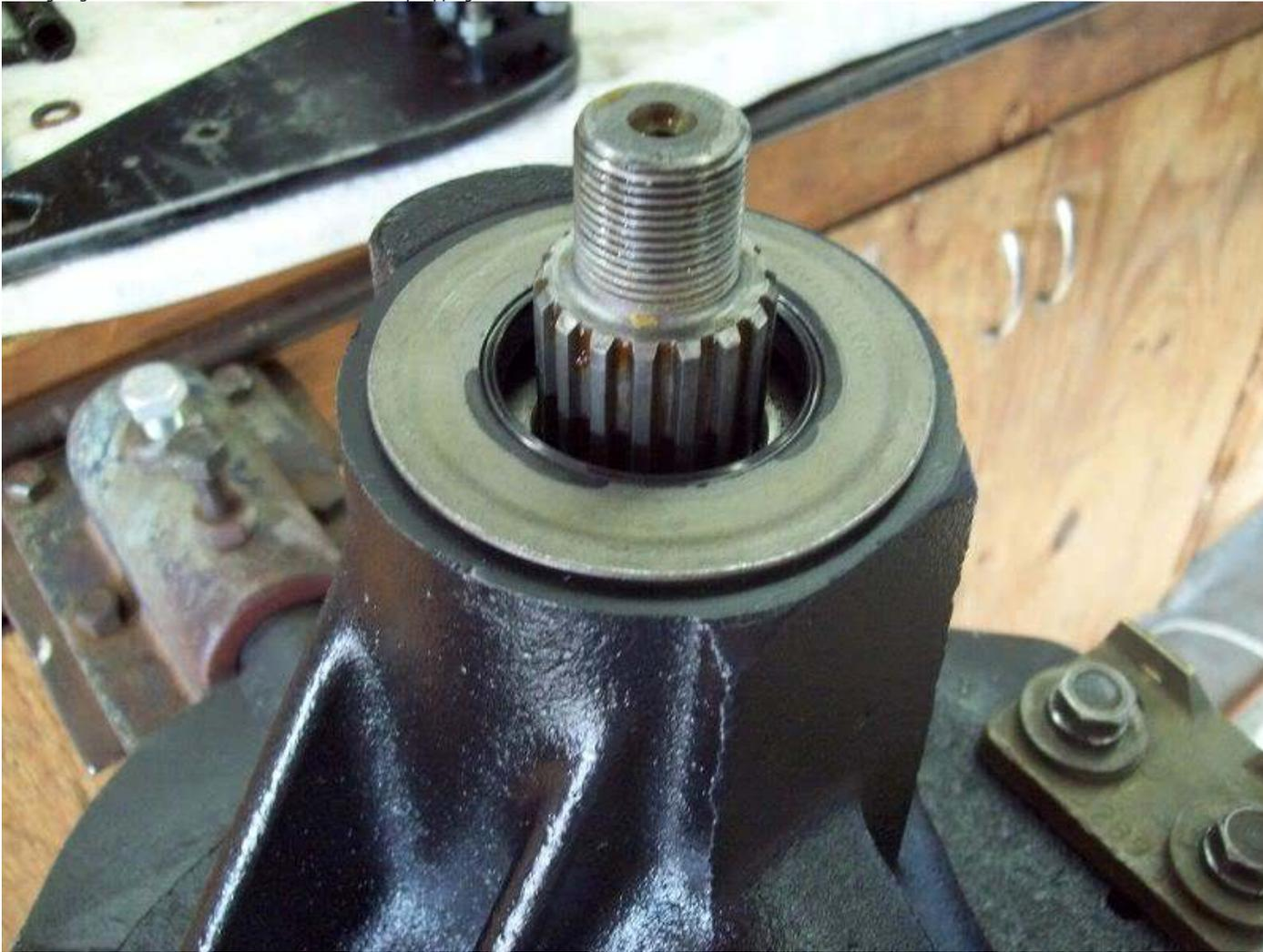
Before putting the yoke back on, I THOROUGHLY clean the splines of the pinion and yoke and paint gasket sealer in the splines of the yoke to seal against an oil leaking through the splines. Put the yoke back on, then the washer and nut.
