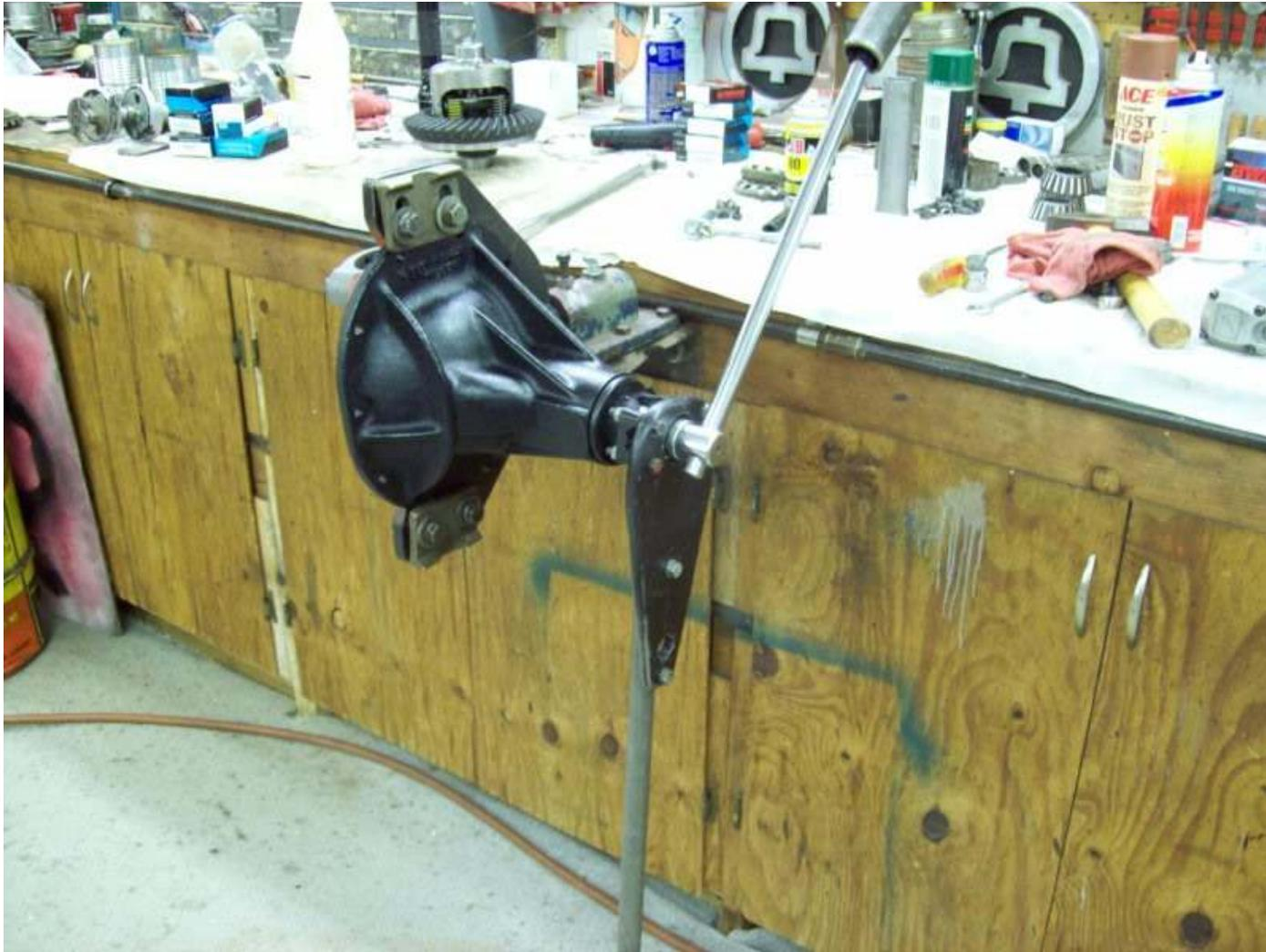
Now bolt the ring gear onto the posi unit and drive the new carrier bearings onto the posi unit. Place the bearing races on the bearings and set the entire assembly into the case. I'm not going into detail here because all of the information for assembly is in the 56 Chevy rearend manual located at the link at the beginning of this article. You can see from the next two pictures where the removed portion of the gusset has provided plenty of clearance for the posi unit.
