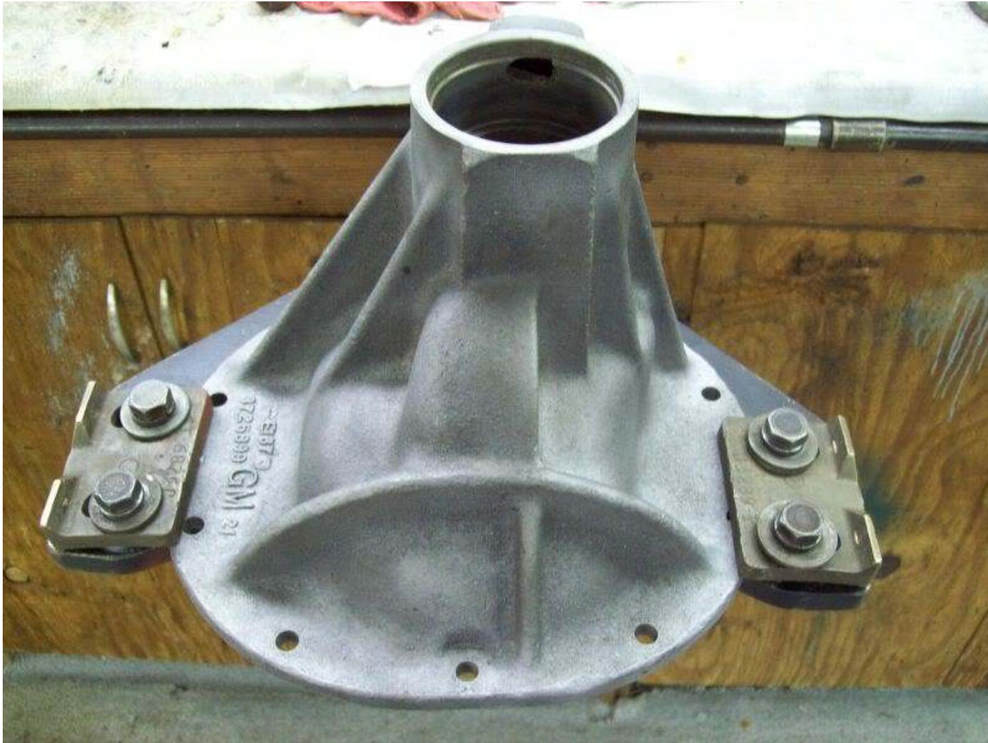
Once the case is cleaned and blasted, it is much easier to read the casting numbers and casting date on the driver side of the case and the ratio code and assembly date (AB 523-May 23) on the passenger side.
