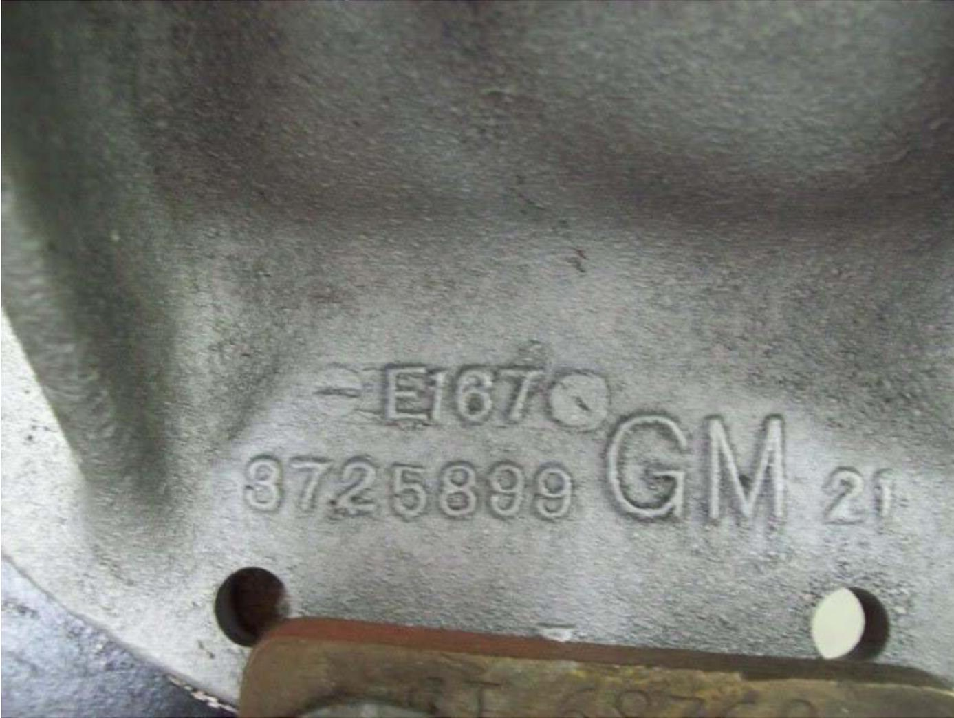
Often the stamped code and assembly date seen below is VERY difficult to find and usually requires thoroughly cleaning down to the bare cast iron.
